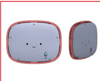
CONVEX MIRROR Shatter resistant mirror, sandwiched between interior gusset and interior fabric layer before binding. Cloud facial features printed on mirror. Snap mirror into mirror holder.
