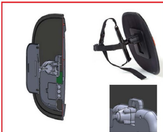
UPDATED BALL JOINT ATTACHMENT Updated Ball Joint attachment from current model to be used. Snapfit to connect joint to housing. Weight from the mirror shouldn't make it move over time on car ride.
